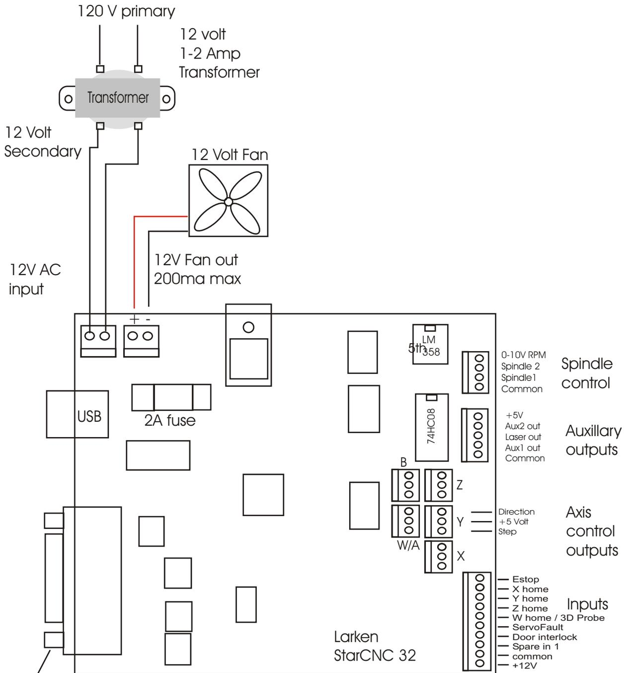
Chassis Grounding required thru mounting plate with Db15 connector
